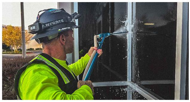
Please keep in mind that this field check method is not good for checking parts that can move, like windows and doors that can be opened and closed. The right way to test for air leakage and water penetration in recently installed windows and doors that can be opened and closed is according to AAMA 502. Also, AAMA 511 is the right standard to use when checking fenestration goods for their ability to stop water from getting through.
