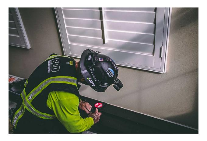
Moisture meters used in conjunction with water intrusion testing
